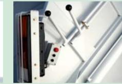
Rear Control Lever (Sliding & Loading Plate)
