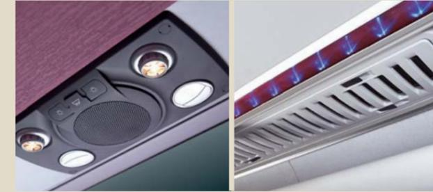
Reading lamp / Air conditioning louver / Air-conditioning return duct grille
