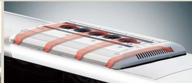
Addition of frame between roof body and air conditioner unit
