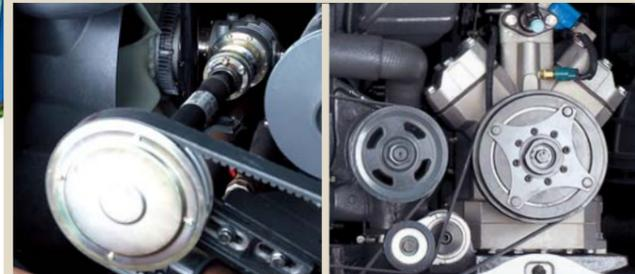
Electro magnetic radiator fan clutch Air-conditioning compressor
