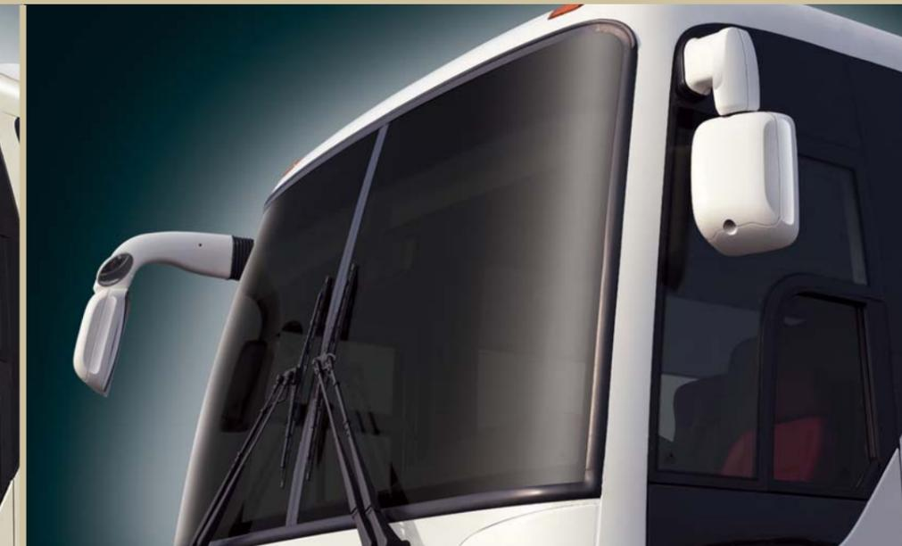
2 piece windshield glass / parallel type wiper / standard outside rear view mirror
