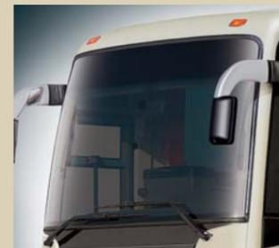
1 piece windshield glass / overlap type wiper / 3 section outside rear view mirror
