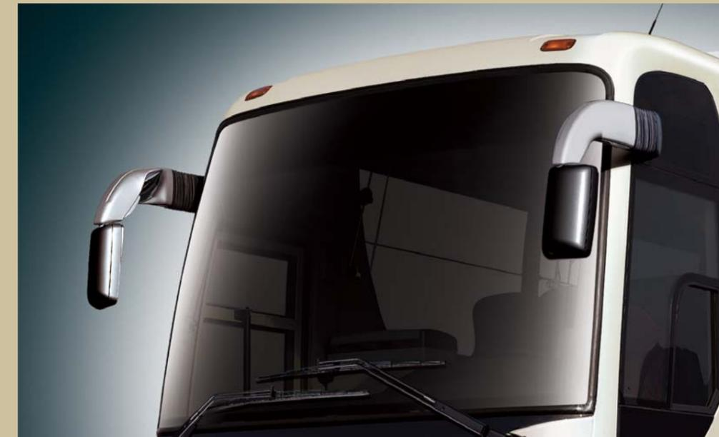
1 piece windshield glass / overlap type wiper / 3 section outside rear view mirror(OPT)
