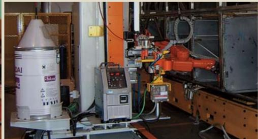
Automatic robot welding of sub structure to side structure
