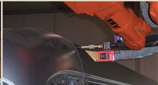
Automatic robot welding of roof structure to side structure
